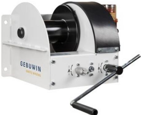
The worm gear winch can be operated both manually and with a cordless drill. A user-friendly winch and often used as a back-up system. If there is a power failure and you want to move a heavy load quickly and effectively, the use of a battery-powered drill offers a solution. The winch is equipped with automatic grease lubrication and a special flexible adaptor to absorb the vibrations of the drilling machine and keep the winch in good condition.
