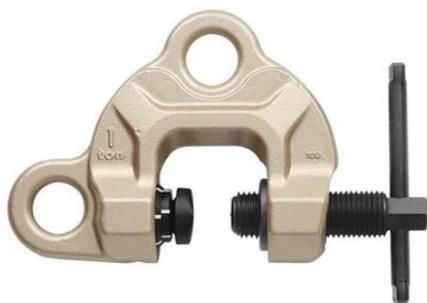
The Tiger CSS safety screw cam clamp with double eye anchor points & safety torque feature is suitable for many applications. This screw cam clamp is for all-purpose uses, such as lifting, lateral pulling and turning over materials. Adequacy of tightening can be visually confirmed by the visual torque safety feature.
