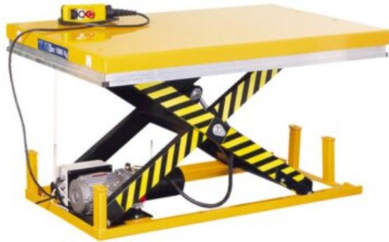
For installation, repairs, packaging etc. Operating voltage 3-phase /380-400 V/50 Hz. Control device (cable) with lifting and lowering functions, as well as emergency stop. Equipped with a protection frame, which prevents the table from lowering, if something gets in between the plates. Electromagnetic valve, the table can not be lowered (it will stop), if a hose breaks. Delivered completely assembled without plug.
