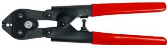
Hand swaging tool is suitable for small 1-1,5 mm soft metal and oval-shaped ferrules used with steel wire ropes. The tool can be used to compress the ferrule and lock the wire rope in place, e.g. when creating a terminal loop. In addition, the tool have integrated wire cutters on the tip of the jaw mechanism. Rubber coating on the handles ensures a firmer grip on the tool.
